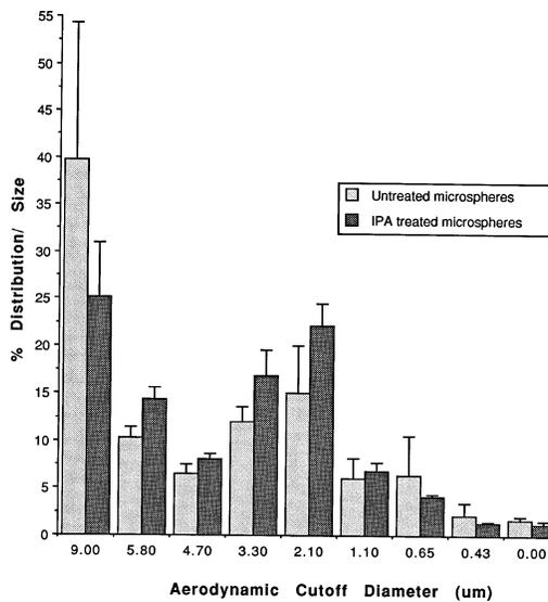
Fig. 2. Radioactivity distribution of <sup>111</sup>In-labeled PLGA microspheres entering the cascade impactor following sampling with a Pfeiffer DPI.
