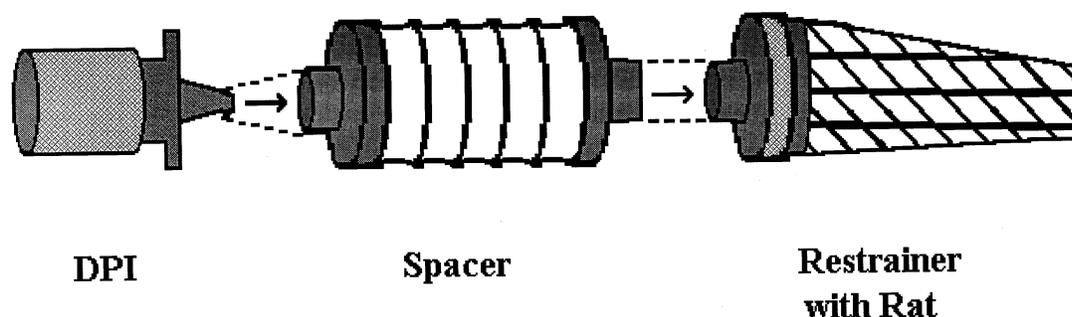
Fig. 1. Schematic of apparatus for administration of powder via DPI to rat.
